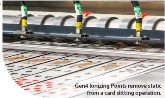
Gen4 Ionizing Points remove static from a card slitting operation.
