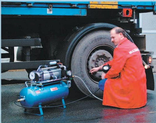
Filling of tyres with 16-bar pressure.
