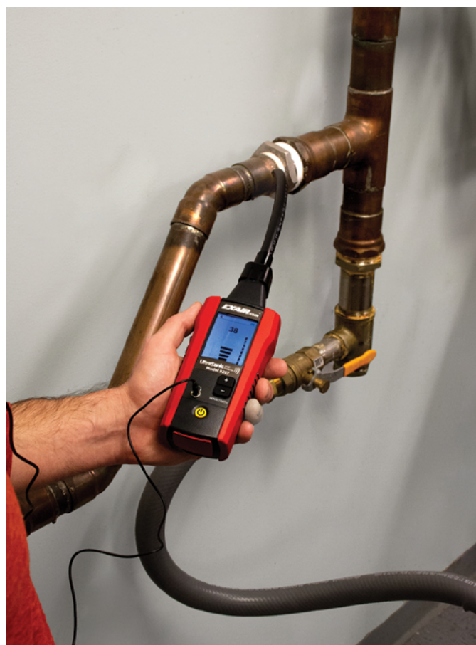
The Model 9207 Ultrasonic Leak Detector with tubular extension quickly pinpoints a costly leak in a noisy industrial environment.
